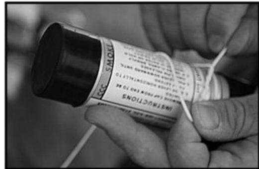
Wrap two turns of the cord around one end the MK-124 flare and tie with a surgeons knot followed by an overhand knot. The turns shall overlap and the knots shall be tied snugly against each other.
